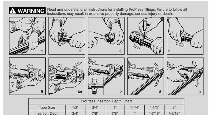
1. Cut copper tubing at right angles using displacement type cutter or fine-toothed steel saw.
